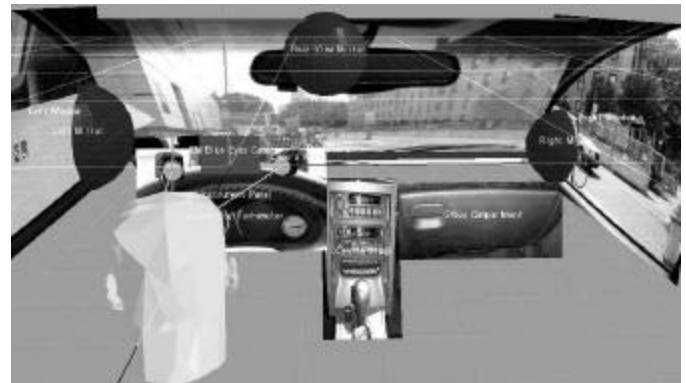
Figure 5. - Cameras track driver's eye position
