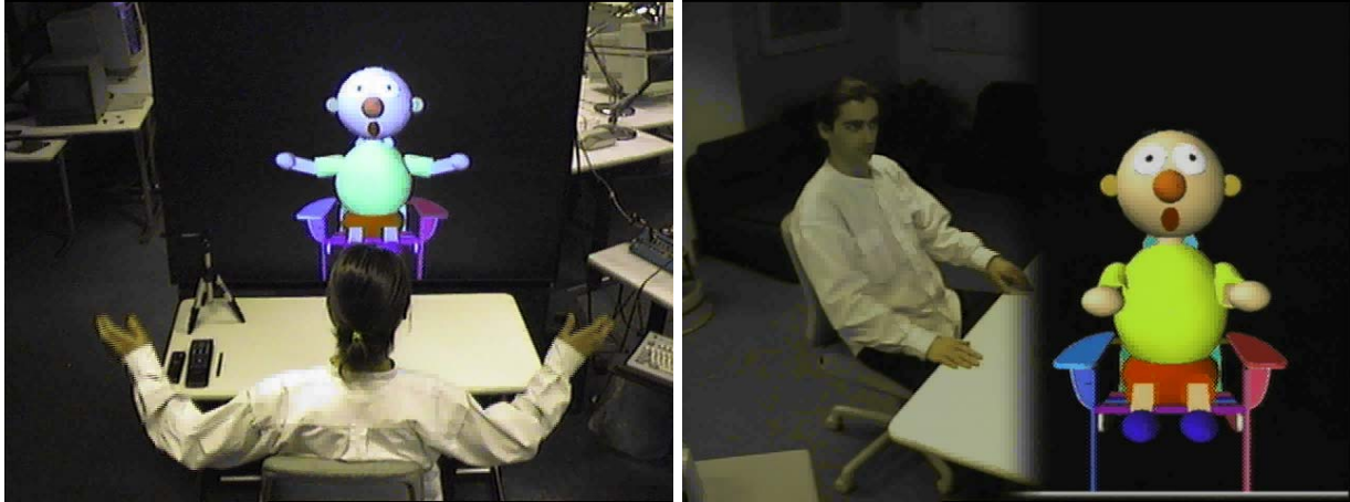
Figure 8: A synthetic character taking direction from a human user who is being tracked in 3-D with stereo vision
